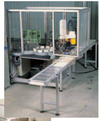
**Above:** Work station for assembling and the computerised inspection of precision guide rails and semi-automatic assembly, inspection and packaging station, with NORCAN frame, housing and conveyor.
