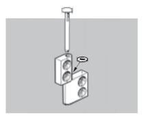
**Double hinge plate - N 1409** with 2 M8 x 20 screws and 2 M8 SC nuts (pin, shaft) for assembly of juxtapositioned hinges on a central 45 mm upright (see fig. 9 below).
